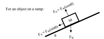
Though here the only problem solved is an object moving on a ramp, this same process is effective on other situations as well. Figure out where the forces are at maximums and minimums, then you will know whether to use sine or cosine for the x and y directions.
