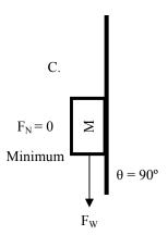
As the surface tilts from 0° to 90°, the amount of  $F_N$  decreases. At 0°  $F_N = F_W$ . At 90° the object falls off the surface, with no friction or  $F_N$  at all.
